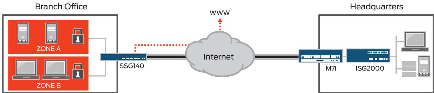
The SSG140 deployed at a branch office for secure Internet connectivity and site-to-site VPN to corporate headquarters. Internal branch office resources are protected with unique security policies for each security zone.
